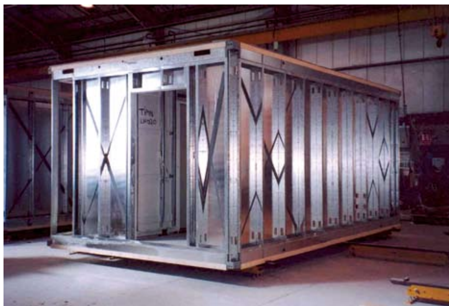
Figure 6.2 Module with load-bearing walls Terrapin
